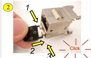
Take the new dust cover. <u>For assembling</u> the new one, place one side into the hinge and pivot the other side while pushing in.
