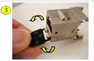
Check both sides are fully inserted and the dust cover is functional and rotates.
