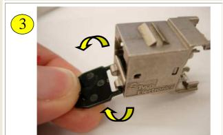
Check both sides are fully inserted and the dust cover is functional and rotates.
