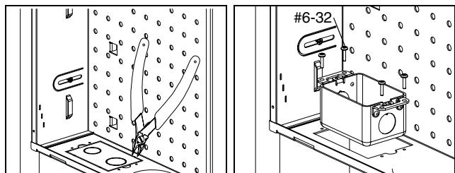
Smaller breakouts are for use with 1/2" and 3/4" conduit.
