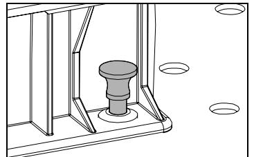
Press plungers down to lock into place.
