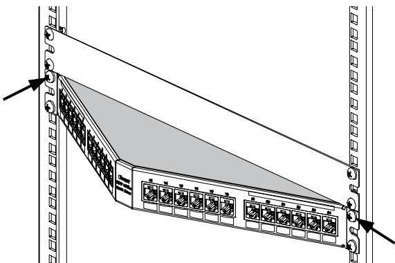
Replace existing M6 screws with the longer screws provided to allow retaining spacers to grip the threads.
