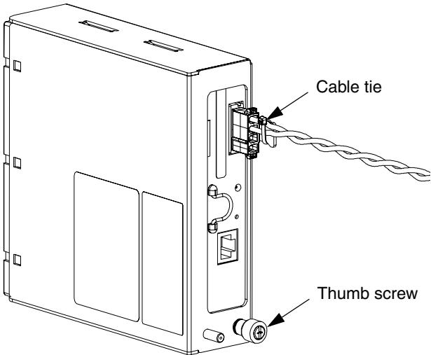
Slide-in and secure the *DPoE* Compact 8 Midspan (*PANDUIT* part no. DPOE8S2XG) or the *DPoE* Modular 8 Port Passive Module (*PANDUIT* part no. DPOEPL8BU) to the Wall Mount Bracket with the thumb screw. Be sure to fasten the power harness to the Wall Mount Bracket with the included cable tie (*PANDUIT* part no. PLT1.5I).
