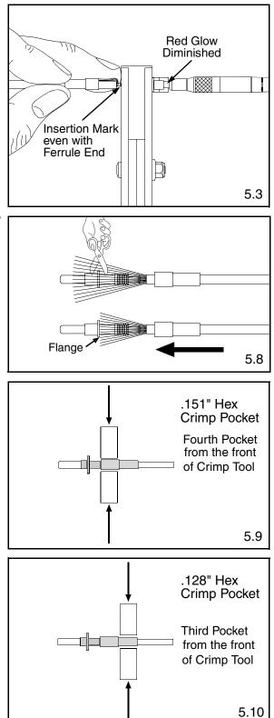
5.8 The fiber jacket should nearly touch the rear of the ferrule assembly.
