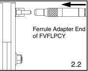
2.2 Remove the dust cap from the connector ferrule in the FCRP5 Crimp Tool. Mate the Ferrule Adapter end of the FVFLPCY to the connector ferrule.
