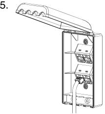
Insert compatible plugs into modules. Align cables 1 per notch on the faceplate as shown above.
