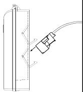
Align notch on module with tab on faceplate.
