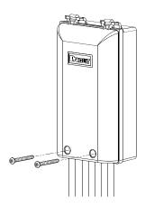
After cables have been aligned, close cover and secure with #6-32 x 1.25" hexagon button head screws or #6-32 x 1.25" combination head screws. For hexagon button head screws use a 5/64" hex key tool.
