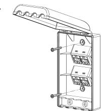
After modules have been installed, align #6-32 x 1" combination head screws with holes as shown above to mount faceplate.
