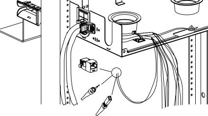
2. Terminate the fibers with an appropriate connector. Mount each connector in the panel.
