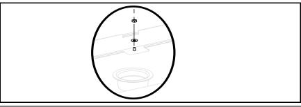
5. Install the hex nut and washer. This will be used to secure the strength member that comes out of the cable.
