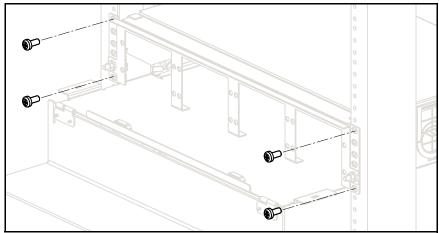
Mount the enclosure to the rack using (4) #12-24 screws.
