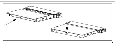
To engage the cover, slide forward until the cover slides under the front tabs then secure in place with #10-32 screw.
