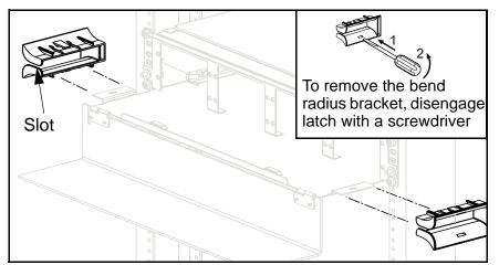
To install the bend radius brackets, slide the bracket onto tab with the slot facing outside then snap in place. (FMD SERIES ONLY)
