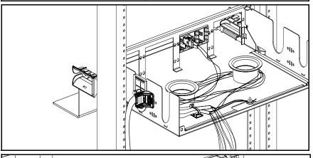
3. Gently loop the excess fiber around the spools. Replace the cover after all fibers are looped around the spools
