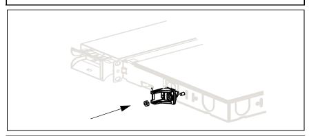
3. Place the strain relief bracket near area where the cable will enter the enclosure. Fasten with #10-32 hex.
