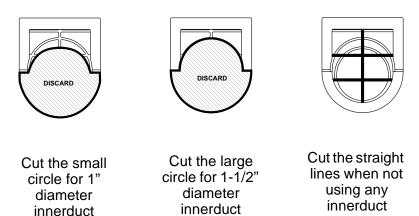
Determine which grommet(s) will be used to bring the cable into the enclosure. Remove the knock-out at entry location of the fiber tray. Install grommet following the proper cutting diagram.
