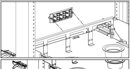
1. Insert the panels into the enclosure as shown. Once mounted, push the latches in to secure the panel.
