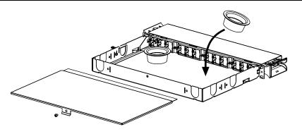
4. Determine where the spools will be located. Remove the liner from the tape on each spool and place them inside the enclosure.
