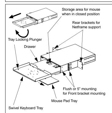
The drawer pulls out 21", rotates 90° counter clockwise and locks in open or closed position with a spring loaded plunger. The mouse pad extends 7". The keyboard tray accepts up to a 18-3/4" keyboard (not included) and wrist pad. The door has magnetic catches with a lanyard support.
