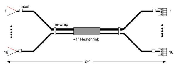
16-channel 18AWG/2-wire Cable Assembly
