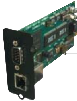
SNMP/Web Card monitors a wide range of UPS information, allowing users to monitor, control, and manage their GXT2 UPS over the network via the Web and SNMP.
