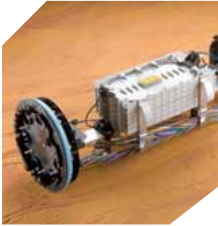
9.5" Dome with Buffer Tube Organizer
