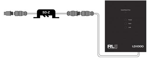
If the SD-Z is being added to an existing system - connected in a chain with other SD-Z devices or cable - undo the appropriate coupling, insert the SD-Z into the chain, and secure all connections.
