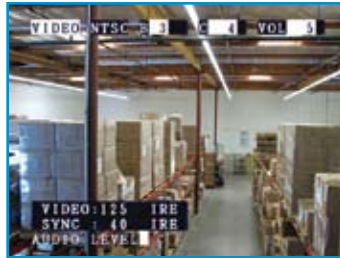
Video and sync level testing in IRE units (NTSC) or millivolts (PAL) and audio level testing with internal speaker and visible level scale. Available only in SecuriTEST PRO model.
