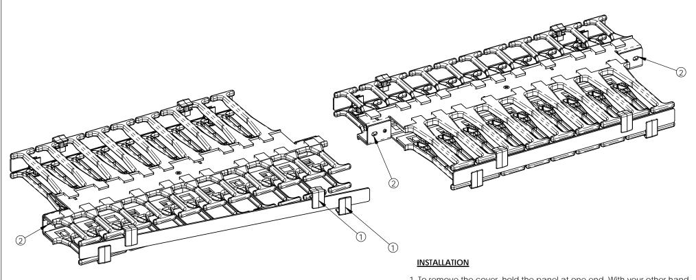
To remove the cover, hold the panel at one end. With your other hand, grasp the upper and lower hinges with your thumb and index finger and pull until hinges release. Repeat this process for the hinges at the other end of the cover.
