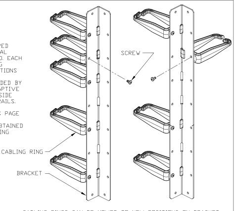
CABLING RINGS CAN BE MOVED TO NEW POSITIONS ON BRACKET AS SHOWN. RINGS CAN BE MOUNTED IN EITHER OF TWO ORIENTATIONS THAT ARE PERPENDICULAR TO ONE ANOTHER.
