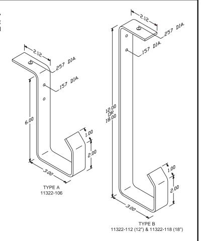
Part Number Dim A Description Type 11322-106 6" Α 6" J-Hook Bracket 11322-112 12" 12" J-Hook Bracket В В 11322-118 18" 18" J-Hook Bracket
