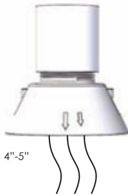
Trim incoming control and power wires to 4-5" for either wall or pendent bracket.
