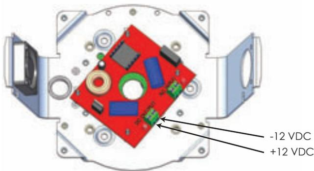
**For 12VDC unit, connect power plug and ET-RJ45 cable to camera.**
