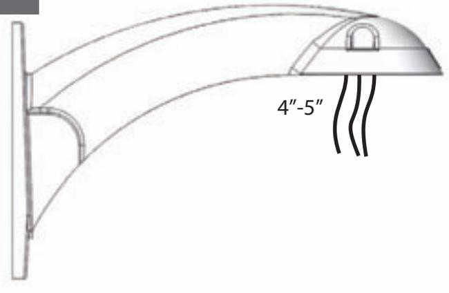
**Trim incoming control & power wires to 4" - 5", for either wall or pendent bracket**
