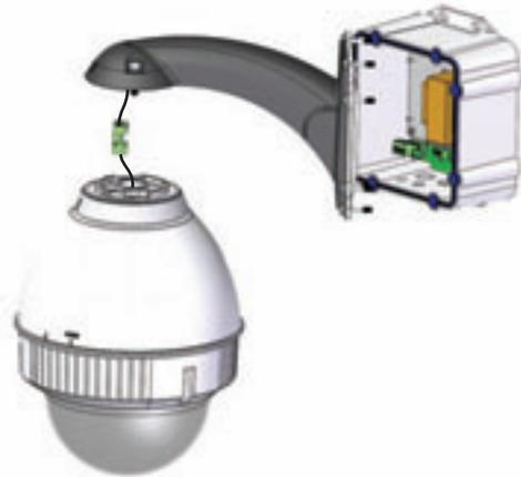
**Additional wires are provided to run power to PB24. Use with connector supplied. Run RJ45 connector through PB24, wall mount, and connect lead from housing.**
