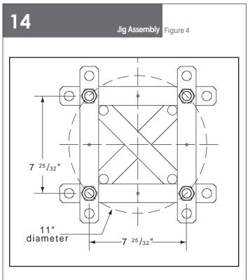
4. Before using the **Anchor Jig** verify that the center to center dimensions between the bolts are even (Figure 4). If not, adjust accordingly. Firmly tighten all **Hex Nuts**.
