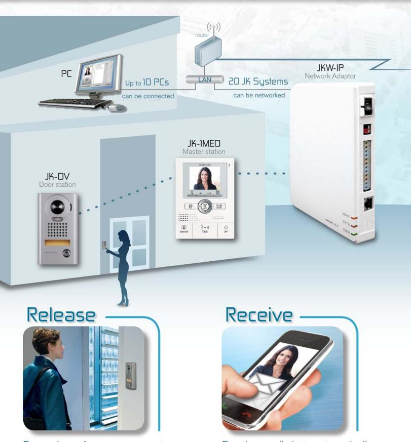
Door release from your computer Confirm identity before allowing entry
