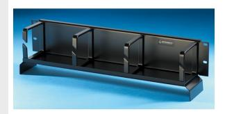
Ortronics bend limiting cable management panels have curved falls that protect against cable crimping and also maintain proper bend radius. The panels are ideal at the top of standard 19" EIA racks. 3.5"H x 3.5"D rings with waterfall, 2 rack units, black.
