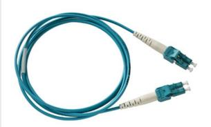
The SpaceSaver line of duplex fiber optic patch cords feature a single 2.4 mm round jacketed cable. These patch cords are available with duplex LC connectors at each end in either A-B or A-A types per the TIA 568 standard and are ideal for high density installations common in data centers and SANs optimizing the available vertical and horizontal cable routing spaces.
