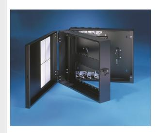
This large volume cabinet accepts our popular Fiber Adapter Panels. The cabinet secures, protects, and organizes single mode or multimode optical terminations. The Cabinet provides interconnect or cross connect facilities between horizontal and backbone inside plant (ISP) or outside plant (OSP) cables. Maximum capacity: 96 Fibers using SC, ST, and FC Adapters, 192 Fibers using MT-RJ and LC Adapters.
