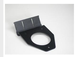
Cable retention bracket providing lances and hook/loop fasteners. Mounts to inside rear of fiber cabinet to provide robust fastening point for incoming backbone cables. Suitable for use with 1U rack mount fiber cabinets.
