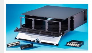
The 3U (5.25" high) fiber cabinet for patching applications is optimized for integration with the Mighty Mo 6 rack system (OR-MM6710, OR-MM6810 & Seismic Rack OR-MM6710S) with 10.5" channel depth. Each fiber cabinet accepts up to nine adapter panels, nine Momentum 1U cassettes. Fiber cabinet can also accept a mix of three 1U and three 2U Momentum cassettes.
