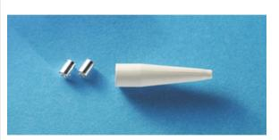
Accessory kit for use in installing SC connectors on 2.4 to 3.0 mm jacketed cables. Kit includes strain relief connector boot using flexible engineering rubber, a cord adapter, a 2.4 mm crimp ring, and a 3.0 mm crimp ring.
