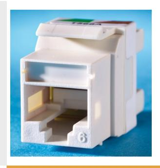
Category 6 Keystone jack, 8-position, 180 degree exit, icon compatible, T568A/B wiring, Fog White Package of 25.TechChoice keystone jacks and modules feature an easy-to-follow universal wiring label and support standard termination using a 110-impact tool. The keystone footprint allows for the greatest flexibility in installation scheduling because its rear insertion into the faceplate allows the technician to complete the termination before and during the construction process. Package of 25.
