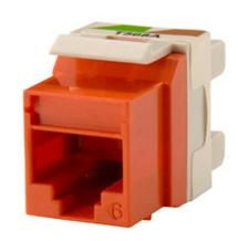
Category 6 Keystone jack, 8-position, 180 degree exit, icon compatible, T568A/B wiring, Orange Package of 25.TechChoice keystone jacks and modules feature an easy-to-follow universal wiring label and support standard termination using a 110-impact tool. The keystone footprint allows for the greatest flexibility in installation scheduling because its rear insertion into the faceplate allows the technician to complete the termination before and during the construction process. Package of 25.
