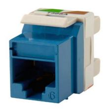
Category 6 Keystone jack, 8-position, 180 degree exit, icon compatible, T568A/B wiring, Blue Package of 25.TechChoice keystone jacks and modules feature an easy-to-follow universal wiring label and support standard termination using a 110-impact tool. The keystone footprint allows for the greatest flexibility in installation scheduling because its rear insertion into the faceplate allows the technician to complete the termination before and during the construction process. Package of 25.
