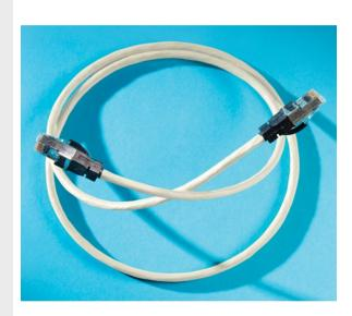
Clarity 6 Shielded, Modular Patch Cord, gray 7', Category 6, four-pair shielded stranded 27 AWG PVC, center tuned with Clarity 6 shielded connecting hardware to provide a significant elevation of channel performance that can be field measured
