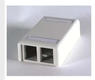
Ortronics TracJack Surface Mount Outlet Boxes accept front-loading TracJack modules and provide snap-on covers and snap-in label fields. Boxes are supplied with screws and double-sided adhesive tape for mounting onto almost any surface. Compatible with Wiremold 2700,2800 and 2900 raceway series.
