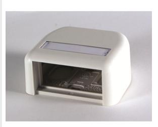
Ortronics Series II Surface Mount Outlet Boxes accept front-loading Series II modules and provide snap-on covers and snap-in label fields. Boxes are supplied with screws and double-sided adhesive tape for mounting onto almost any surface. Compatible with Wiremold 2700, 2800 and 2900 raceway series.
