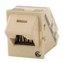
Clarity 6 Angled TracJack, ETL verified to TIA Category 6 component specification, is front-loading and front removable. New universal T568A/B wiring label and tapered wiring towers simplify termination. Center tuned to Clarity 6 patch cords for optimum performance.
