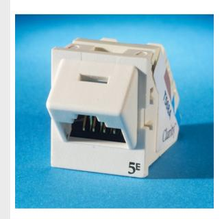
Clarity 5E Angled TracJack, ETL verified to TIA Category 5e component specification, is front-loading and front removable. New universal T568A/B wiring label and tapered wiring towers simplify termination. Center tuned to Clarity 5E patch cords for significant performance above Category 5e.
