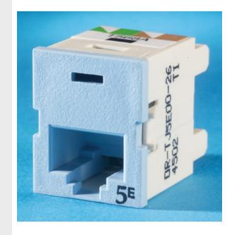
Clarity 5E TracJack, ETL verified to TIA Category 5e component specification. Front-loading and front removable. New universal T568A/B wiring label and tapered wiring towers simplify termination. Center tuned to Clarity 5E patch cords for significant performance above Category 5e
