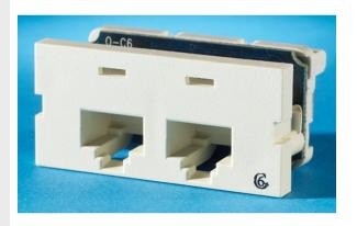
Clarity 6 Series II module two jack ports (1 unit), ETL verified to TIA Category 6 component specification. Front-loading and front removable. New universal T568A/B wiring label and tapered wiring towers simplify termination. Center tuned to Clarity 6 patch cords for optimum performance. 180°
