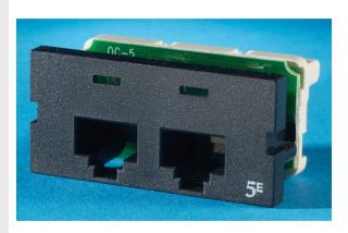
Clarity 5E Series II module two jack ports (1 unit), ETL verified to TIA Category 5e component specification. Front-loading and front removable. New universal T568A/B wiring label and tapered wiring towers simplify termination. Center tuned to Clarity 5E patch cords for optimum performance.
