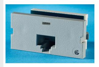
Clarity 6 Series II module one jack port (1 unit), ETL verified to TIA Category 6 component specification. Front-loading and front removable. New universal T568A/B wiring label and tapered wiring towers simplify termination. Center tuned to Clarity 6 patch cords for optimum performance.
