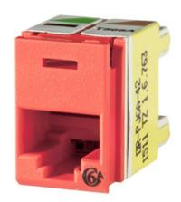
Clarity 6A patch panel jacks, rear load into patch panels and exceed Category 6a component specifications. Rear load positive latch design, secures mounting of the jack into the patch panel. Universal T568A/B wiring label and tapered wiring towers simplify termination.
