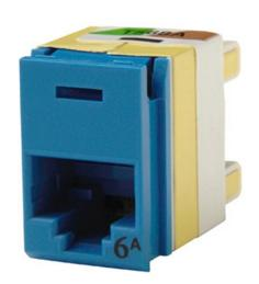
Clarity 6A panel jacks, rear load into panels and exceed Category 6A component specifications. Rear load positive latch design, secures mounting of the jack into the panel. Universal T568A/B wiring label and tapered wiring towers simplify termination.
