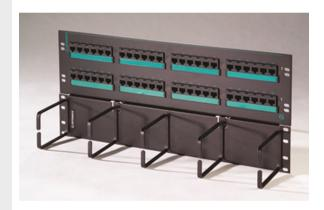
Clarity 5E 48-port standard density patch panel with hinged cable management panel is component compliant to TIA/EIA Category 5e performance requirements. It occupies 4 rack units and measures 19" x 8.75". Jacks are grouped in six-port modules. It is part of the Clarity 5E link and channel solution that provides significant installed performance headroom.
