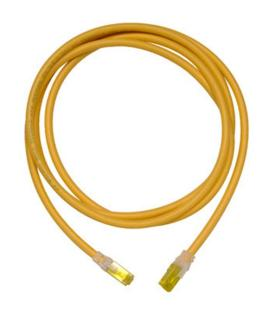
Clarity 10G modular patch cord, yellow, 15', 10 Gigabit, four-pair UTP stranded 26 AWG PVC/CM, center tuned with Clarity connecting hardware for optimum installed performance using Ortronics Paralign 2 pair-positioning technology.
