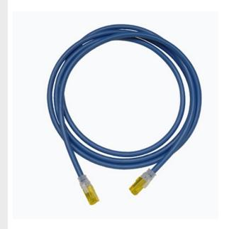
Clarity 10G modular patch Cord, blue, 9', 10 Gigabit, four-pair UTP stranded 26 AWG PVC/CM, center tuned with Clarity connecting hardware for optimum installed performance using Ortronics Paralign 2 pair-positioning technology.
