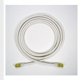
Clarity 10G modular patch cord, white, 5', 10 Gigabit, four-pair UTP stranded 26 AWG PVC/CM, center tuned with Clarity connecting hardware for optimum installed performance using Ortronics Paralign 2 pair-positioning technology.
