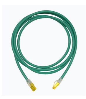
Clarity 10G modular patch cord, green, 3', 10 Gigabit, four-pair UTP stranded 26 AWG PVC/CM, center tuned with Clarity connecting hardware for optimum installed performance using Ortronics Paralign 2 pair-positioning technology.
