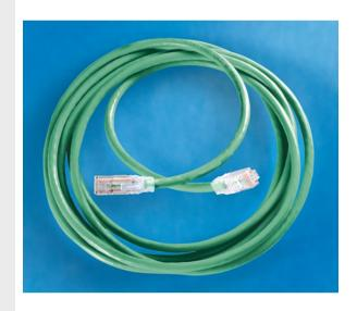
Clarity 5E Premium Category 5e Modular Patch Cord, green, 25', Category 5e, four-pair UTP stranded 24 AWG PVC/CM, center tuned with Clarity 5E connecting hardware for optimum Category 5e installed performance using Ortronics Paralign 2 pair-positioning technology
