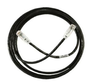
Clarity 5E Premium Category 5e Modular Patch Cord, black, 5', Category 5e, four-pair UTP stranded 24 AWG PVC/CM, center tuned with Clarity 5e connecting hardware for optimum Category 5e installed performance using Ortronics Paralign 2 pair-positioning technology.
