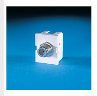
TracJack Module provides a single F-connector coupler F/F with under .2dB of insertion loss at 2GHz (1/3 the loss of standard models). TracJack is a versatile single jack solution in a front-load footprint which allows a choice of up to six jacks/connectors to fit in a single gang plate
