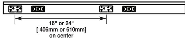
**NOTE:** Top channel Should be reserved for data to provide highest capacity and bend radius. Standard forward facing faceplates can be intermixed with prewired, but are subject to location restrictions due to the location of downward facing data. Consult factory for recommended locations.
